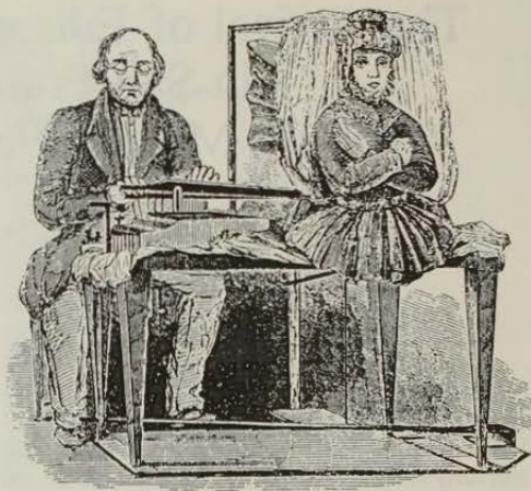
FIGURE 2. The Euphonia, or Speaking Machine, exhibited in London the summer of 1846. From The Illustrated London News (August 6, 1846, 96). The levers are located at one end of the small table, with the treadle below. The bellows are located behind the corseted waxen lady, not beneath the table. The machine is positioned horizontally—not vertically, as demonstrated in San Francisco.
